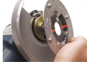
Place the backing plate on your angle grinder.
