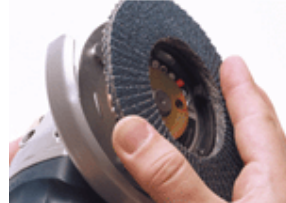
Match the CMT "loading" to the backing plate.
