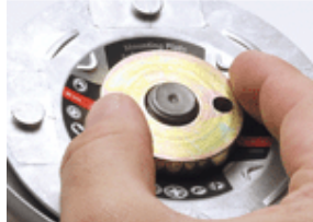
Use your standard locking nut to fasten the backing plate in place.
